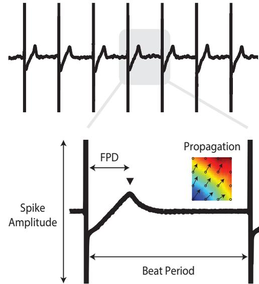
**Figure 1.** Top: Maestro MEA recording of cardiomyocyte activity. Bottom: The Maestro's fast data collection rate (12.5 kHz), sensitive microvolt resolution, and industry-leading electrode density enables collection of numerous cardiomyocyte activity metrics. This figure shows measures commonly used in cardiac safety studies.
